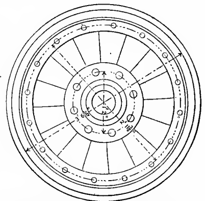
Fig. 5320. TEAK-WOOD-CENTER WHEEL. Tire fastened with Mansell Rings. Largely in use in England.
